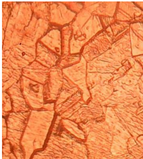
Figure 14. Micrograph of C-110 Copper specimens before exposure
