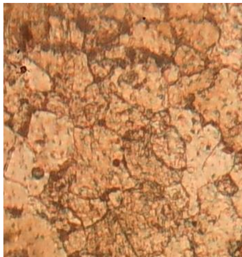
Figure 11. Micrographs of C-1020 mild steel specimen before exposure
