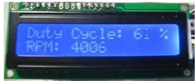
Fig 6: LCD display showing speed for set duty cycle
