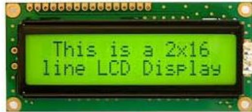
Fig.1. LCD Display
