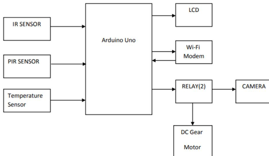
**Fig 1: Block Diagram of IOT based Border Surveillance System**
