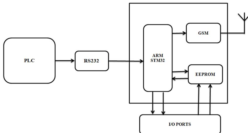
**Fig 2:** Hardware Block diagram for smart factory 4.0.
