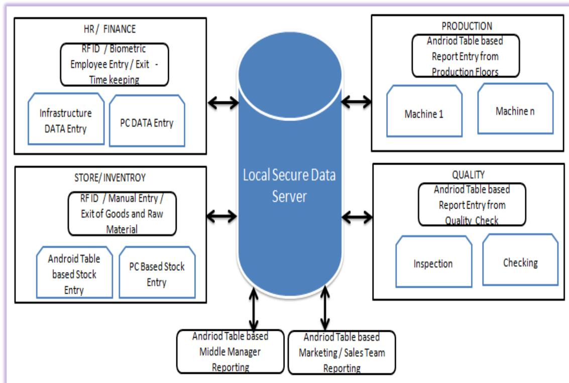
**Fig 1:** System Block diagram for smart factory 4.0.
