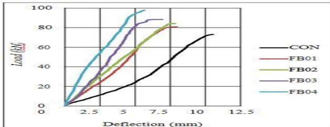
**Fig.4:** Load Vs deflection curve for strengthened RC beams
