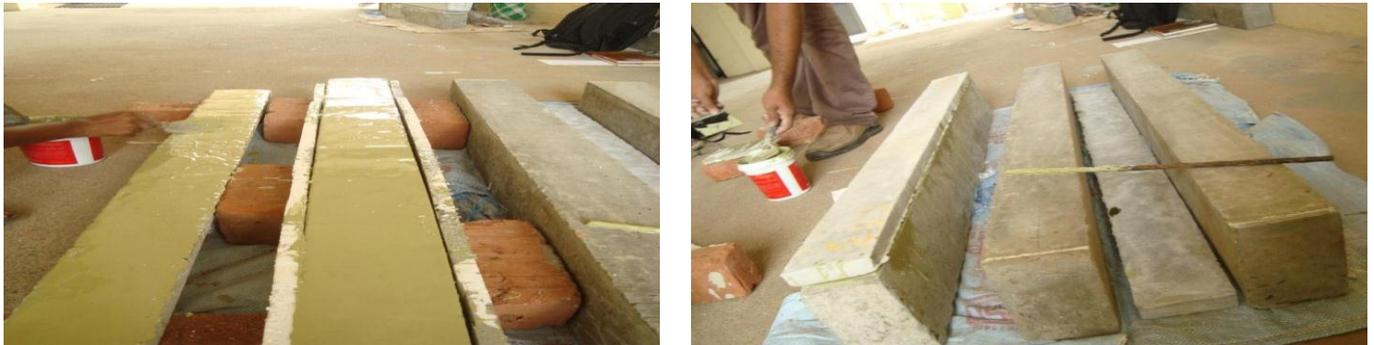
**Figure 3:** Application of epoxy resin on RC beam, laminate and Strengthened RC beam
