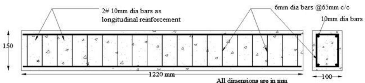
Figure 2: RC Beam Design
