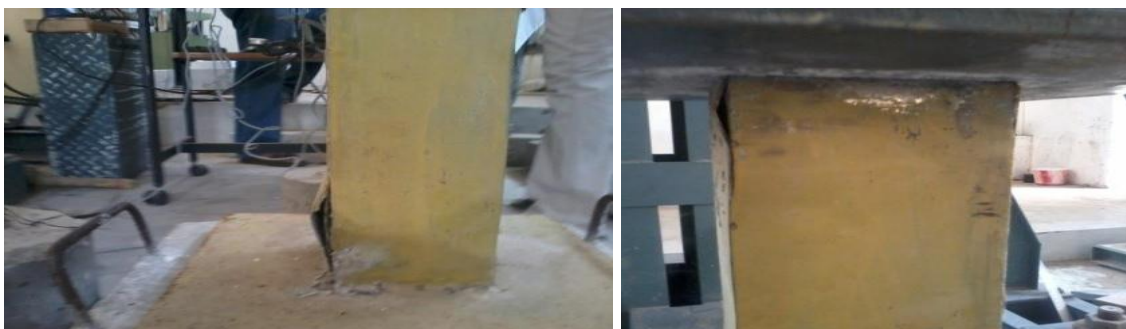
Fig.6.2. Failure patterns of composite columns
