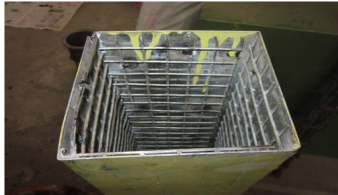
Fig 4.2. Steel column with wire mesh welded inside
