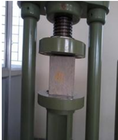
Fig.5.1. Compressive strength test on concrete cube
