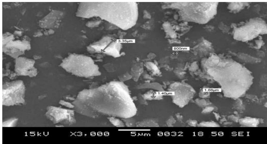
**FIG 2.3: SEM MICROGRAPH OF CARBON ON SILICA**
