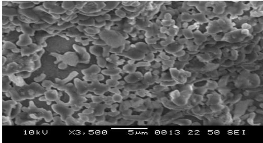
**FIG 2.2: SEM MICROGRAPH OF A TYPICAL SILICA EXAMPLE**
