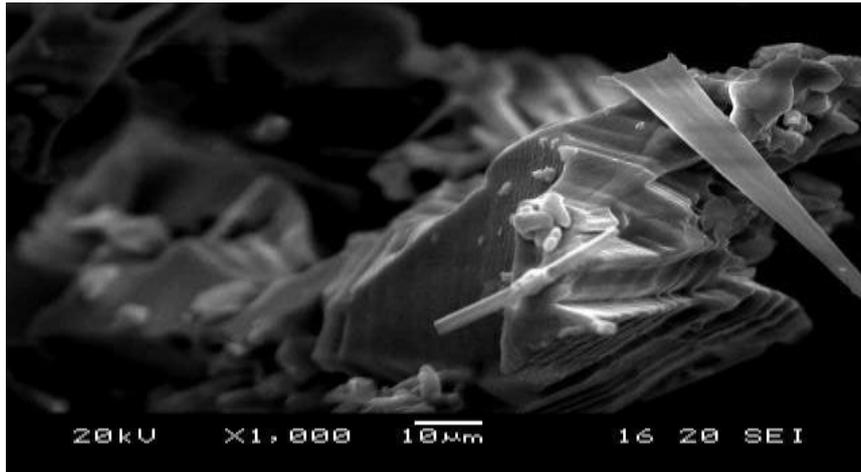
**FIG 2: SEM IMAGE SHOWS SILICA PARTICLES OBTAINED BY USING HCL IN ACID WASHING**
