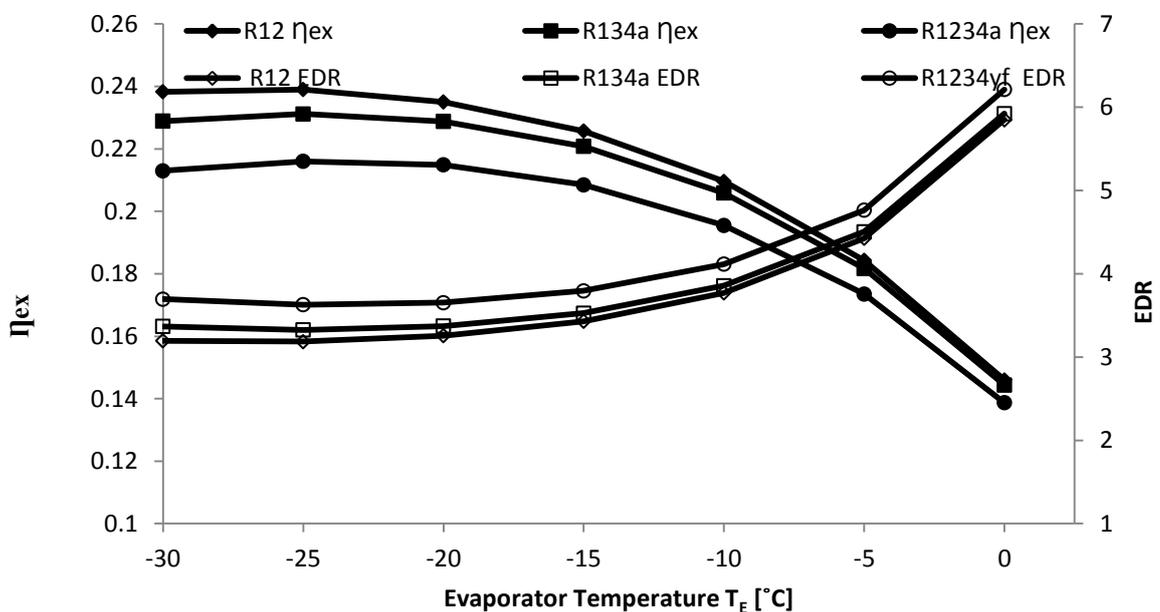
Fig. 3.2 Variation in  $\eta_{ex}$  and EDR with evaporator temperature
