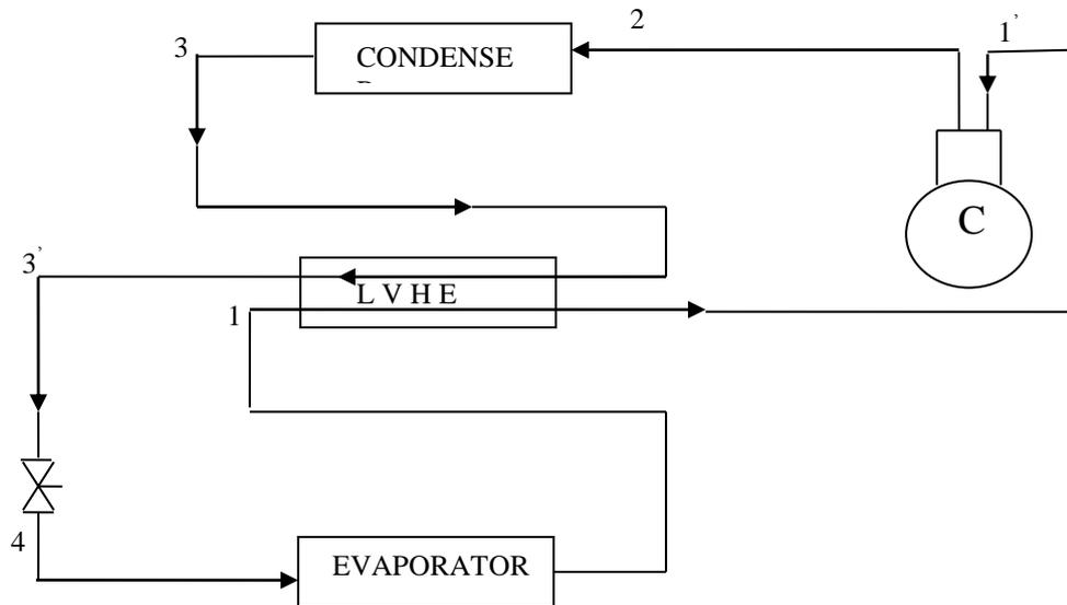
**Fig. 2.1: Schematic diagram of vapour compression system with LVHE**
