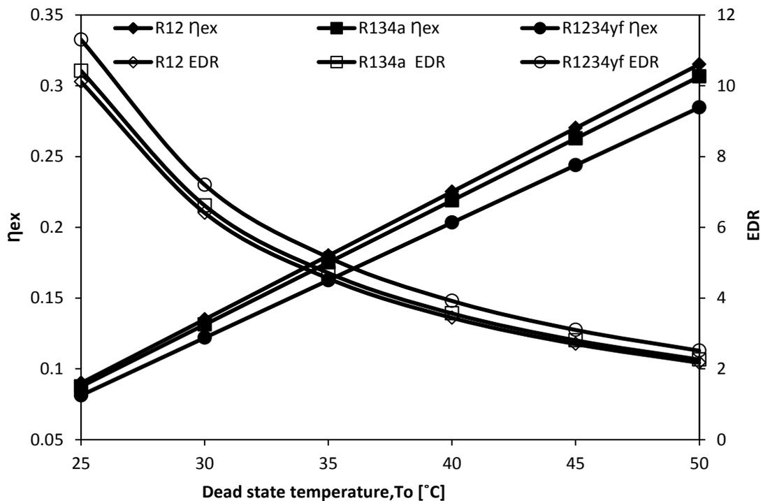
Fig.3.3 Variation in value of exergetic efficiency with dead state temperature
