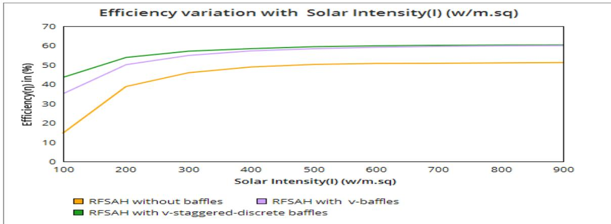
The above graph shows that the efficiency varies with solar intensity (I) only up to 400(w/m.sq.) , and after this the efficiency becomes almost asymptote for all three types of variations in Return flow solar air heater. For Return flow solar air heater with v-staggered-discrete baffles the maximum efficiency is nearly 60% for a mass flow rate of 0.03kg/sec compared to 59% for Return flow solar air heater with v- baffles for same mass flow rate
