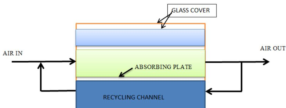
**Sopian et al. [5]** used a heater based on sun with some porous medium in second channel. He conducted indoor experiments and deduced that 2-pass solar heater for air with some porous medium in second channel has thermal efficiency ranging 60% to 70% i.e. about 10% to 20% excessive than that one without any porous medium
