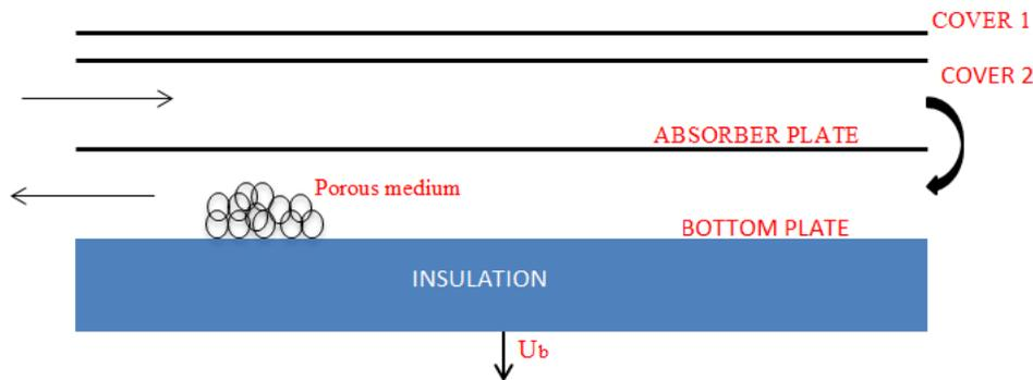
**Naphon[6]** examined theoretically the characteristics of heat transfer and performance associated with 2-pass flat sun oriented air heater both with and also without any porous media. The mathematical model presented in this examination of designed 2-pass single solar air collector along with some porous media is established from model presented by researchers Naphon and Wijesundera
