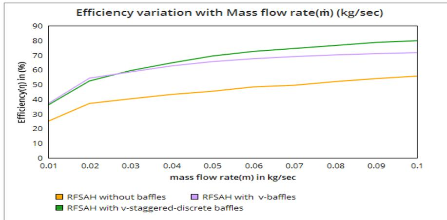
From the above graph we can see the variation of efficiency with change in mass flow rate for different arrangements of return flow solar air heater. It is clearly visible that efficiency increases significantly on application of baffles on absorber plate. For both flat plate return flow solar air heater and Return flow solar air heater with v-baffles the efficiency increases with mass flow rate to certain point and then becomes nearly constant.
