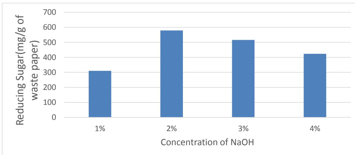
Fig 3.1.1: Reducing Sugar (mg/g of waste paper) versus concentration of NaOH in the Microwave treated sample
