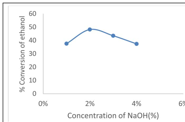
Fig 3.4.1: Variation of % Conversion of Ethanol for sonication assisted sample
