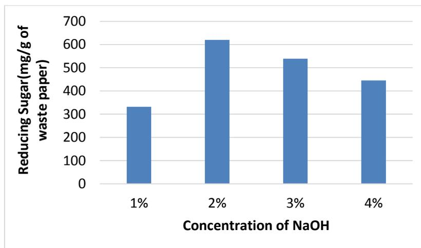
Fig 3.1.2: Reducing Sugar (mg/g of waste paper) versus concentration of NaOH in the Sonication treated sample
