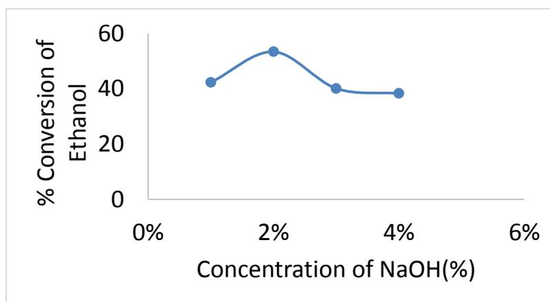
Fig 3.4.2: Variation of % Conversion of Ethanol for sonication assisted sample
