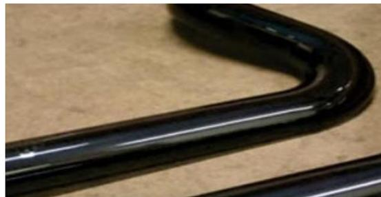
Figure.2. Carbon steel coated with polyurethane paint
