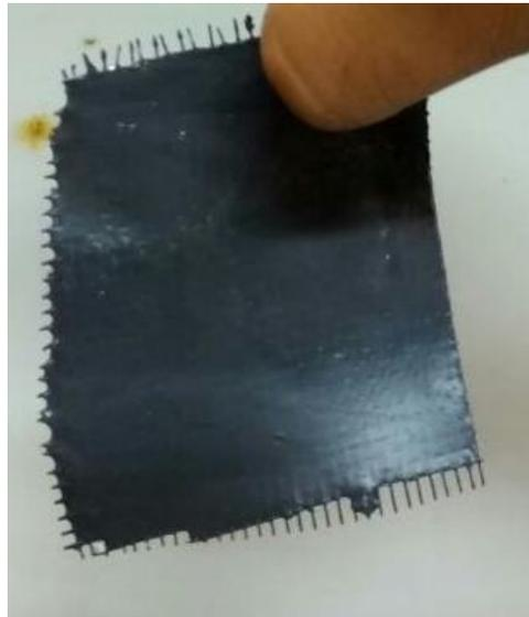
Fig. 3.3.1: Cathode after fabrication using phase inversion
