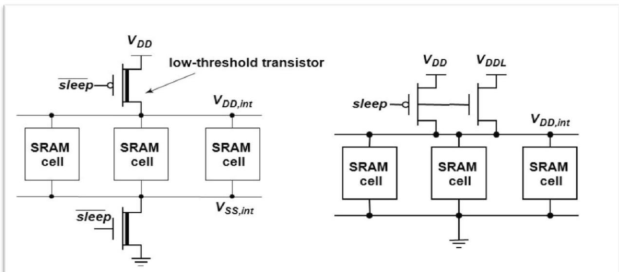
Figure 1.4 Leakage Suppression Techniques.
