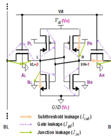
Figure 1.2 Different components of SRAM cell leakage
