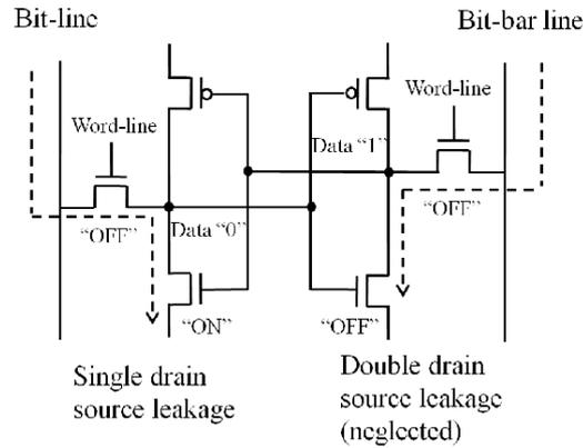
Figure 1.5 Sub-Threshold leakage control technique
