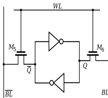
Figure 1.3 6T-SRAM cell
