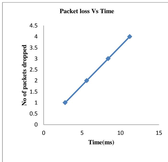
Fig 2(d) : Packet loss Vs Time for Passes algorithm
