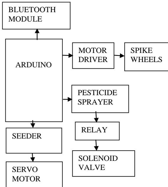
Fig:1 Block Diagram of AGRIBOT
