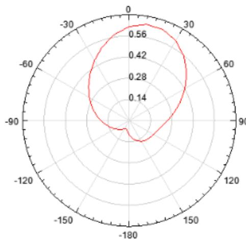
Fig. 4. (c) Radiation pattern of unslotted fractal UC-EBG
