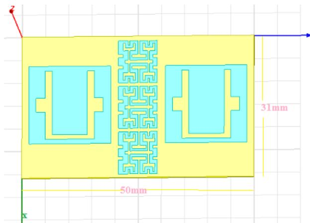
Fig.3.Modified U-slot microstrip patch antenna
