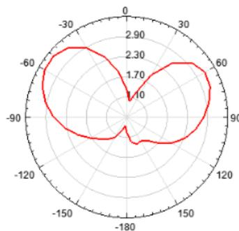
Fig. 5(c). Radiation pattern for U-slotted MSA
