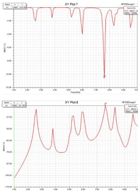
Fig. 4. (a) Simulated result of return loss for unslotted fractal UC-EBG (b) Simulated result of isolation for unslotted fractal UC-EBG
