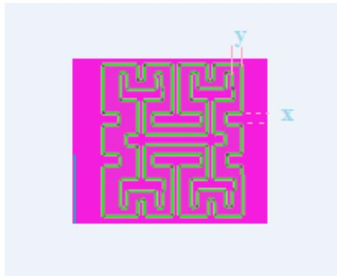
Fig :1. Geometry of the fractal UC-EBG unit cell
