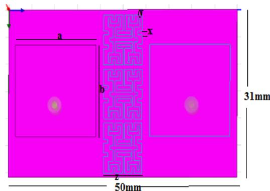
Fig.2. Unslotted fractal UC-EBG structure
