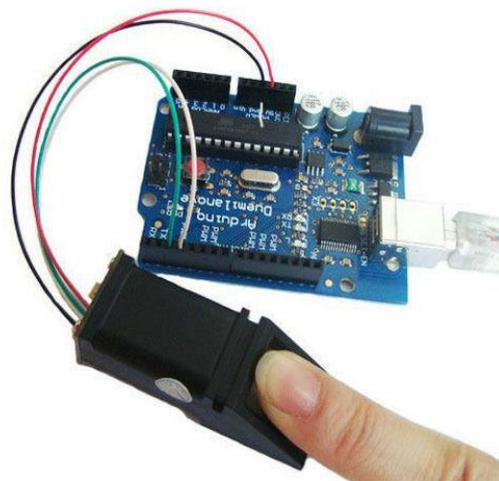
Figure 3: Diagram for arduino with finger print scanner
