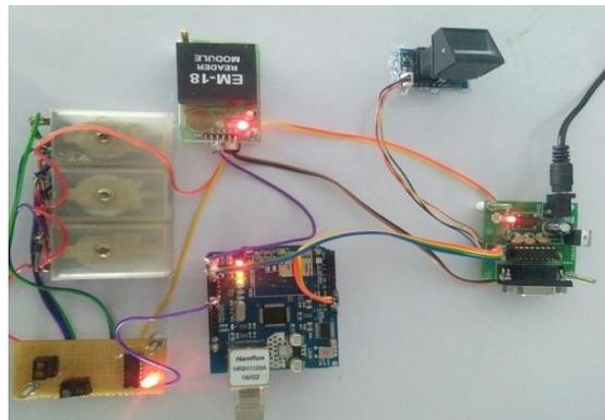
Figure 2: Electronic circuit Breaker with fingerprint scanner
