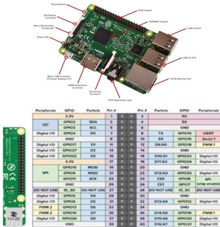
Fig (2): Raspberry Pi3 and GPIO pins
