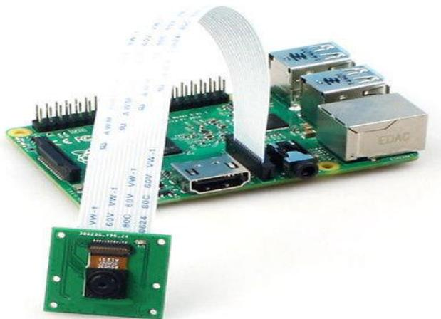
Fig (3): Raspberry Pi-3 with Camera interface.
