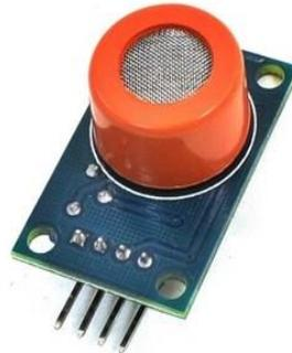
Fig 5: Alcohol Sensor
