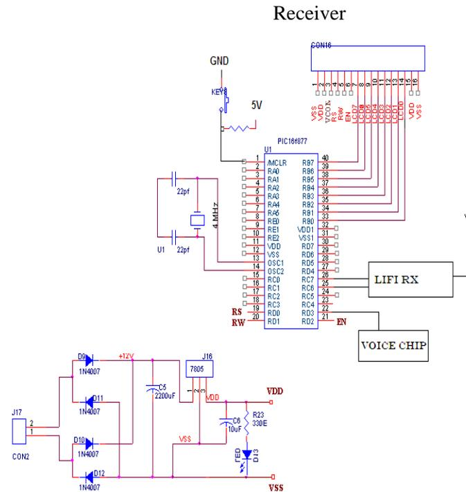
Figure 6. Circuit Diagram of Proposed system
