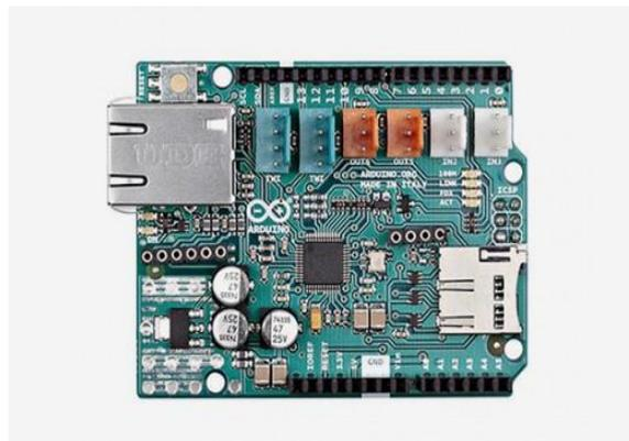
Figure 5: Ethernet shield
