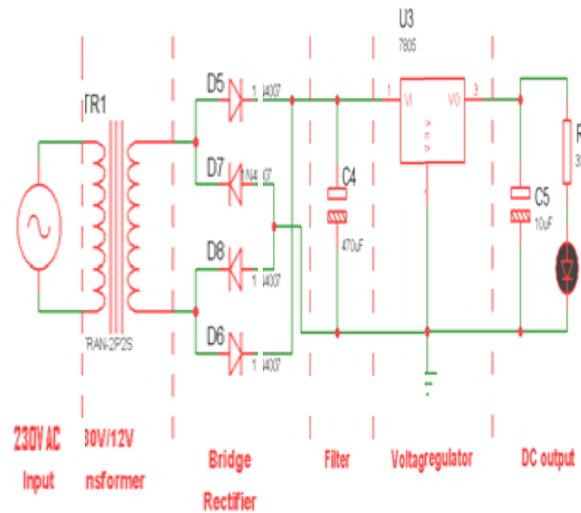
Figure 2: Power supply unit
