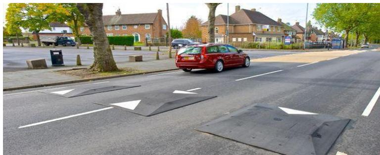
Figure 2. Adjustable speed breaker
