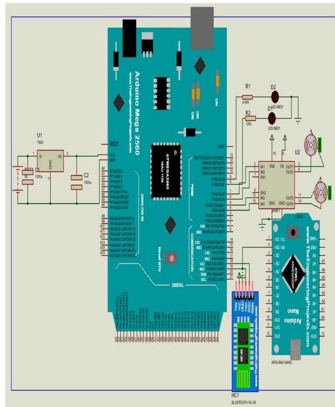
Fig. 6. Circuit Diagram of Wheelchair
