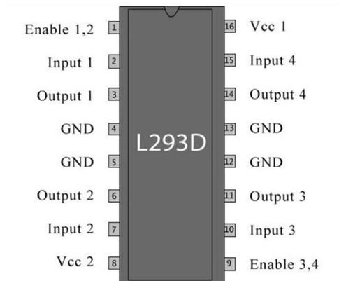
Fig. 7. L293D Pin Configuration
