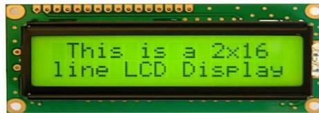
An LCD consists of two glass panels, with the liquid crystal material sandwiched in between them. The inner surface of the glass plates are coated with transparent electrodes which define the character, symbols or patterns to be displayed. Polymeric layers are present in between the electrodes and the liquid crystal, which makes the liquid crystal molecules to maintain a defined orientation angle.
