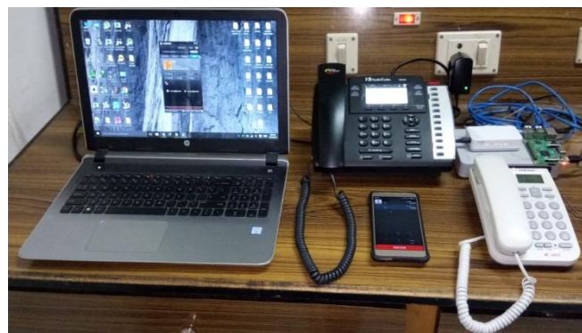
Fig. 20. Hardware setup of proposed IP-PBX system
