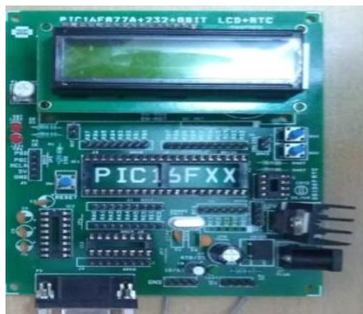
Fig .5.PIC Microcontroller
