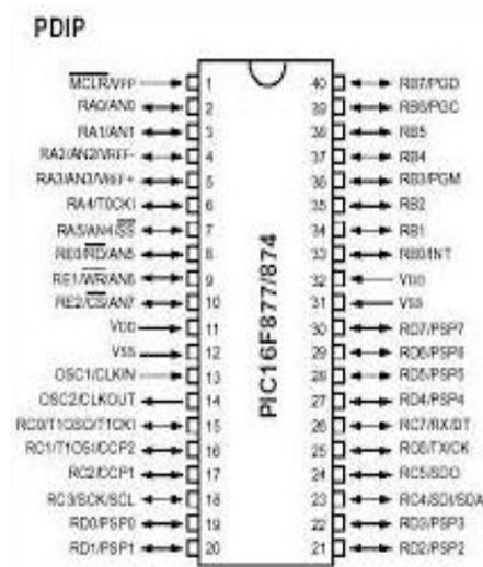
Fig.6.Pin diagram of PIC16F8XX
