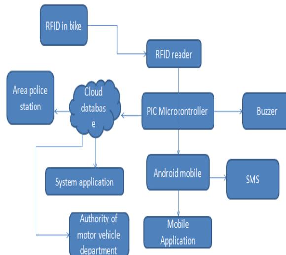
Fig .2. Proposed System Block Diagram
