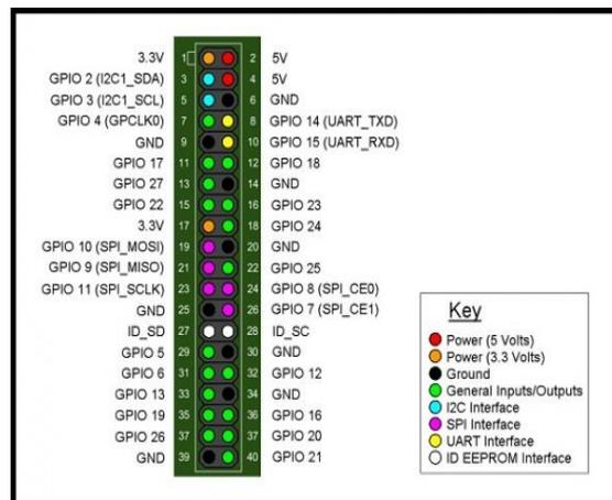
Fig 4: Pin Configuration
