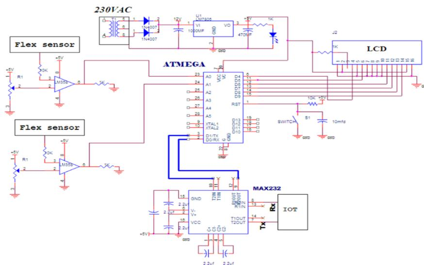
Fig 2. Transmitter Circuit
