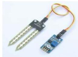
Fig.3 Soil moisture sensor
