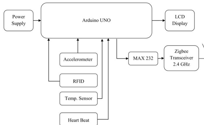
Transmitter Block Diagram
