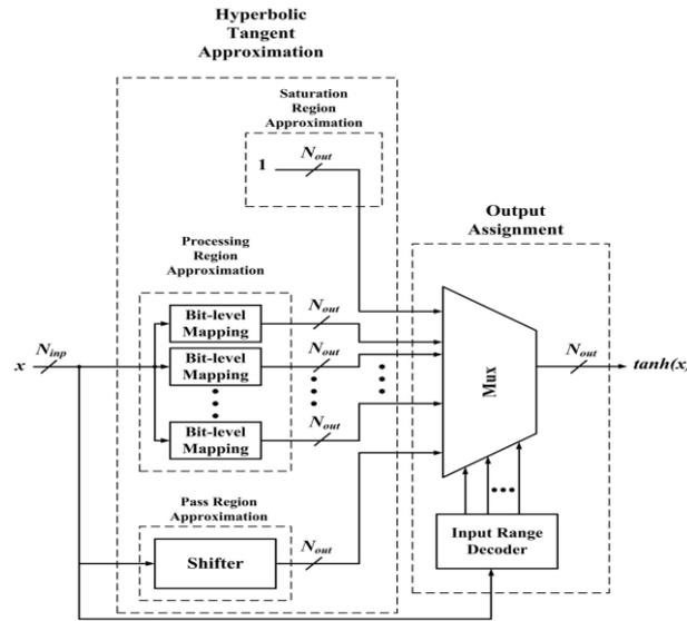
Fig.3.1. Block diagram of proposed structure
