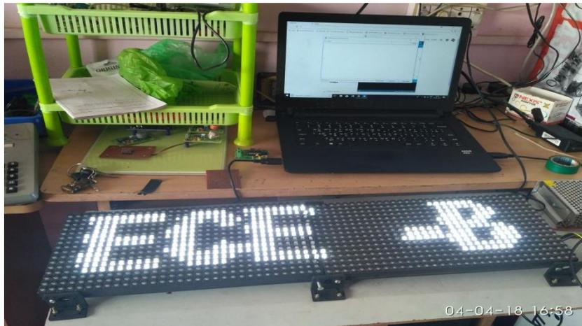
Fig 8. Hardware display of wireless notice board
