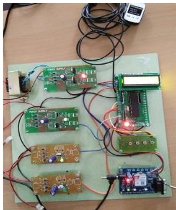
Fig.3. Underground cable fault distance locator
