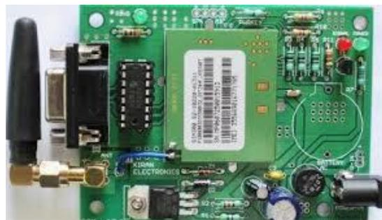
Fig.2. GSM Module
