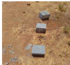
Fig 3. Ambient curing of concrete
