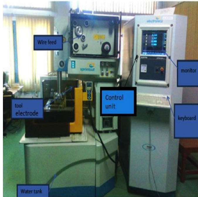
Figure 1: Experimental setup of WEDM
