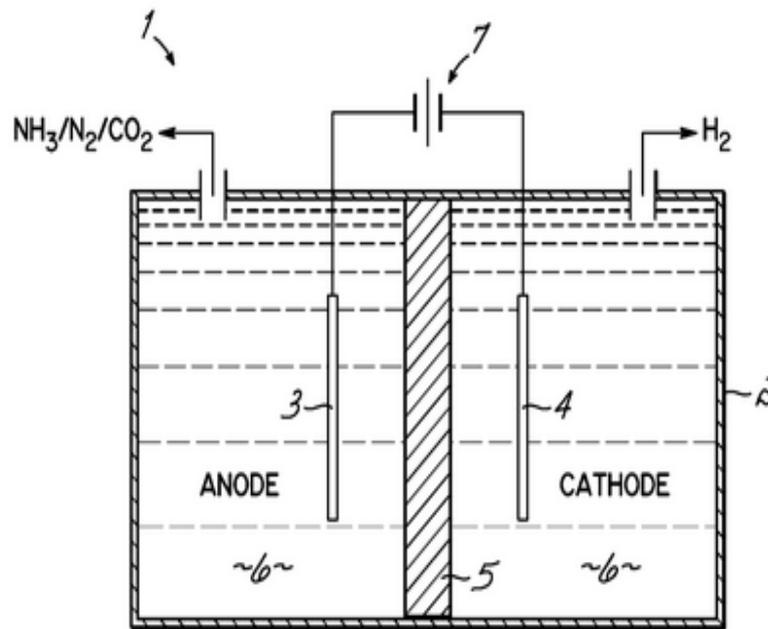
Fig 2: Scheme of urine electrolysis
