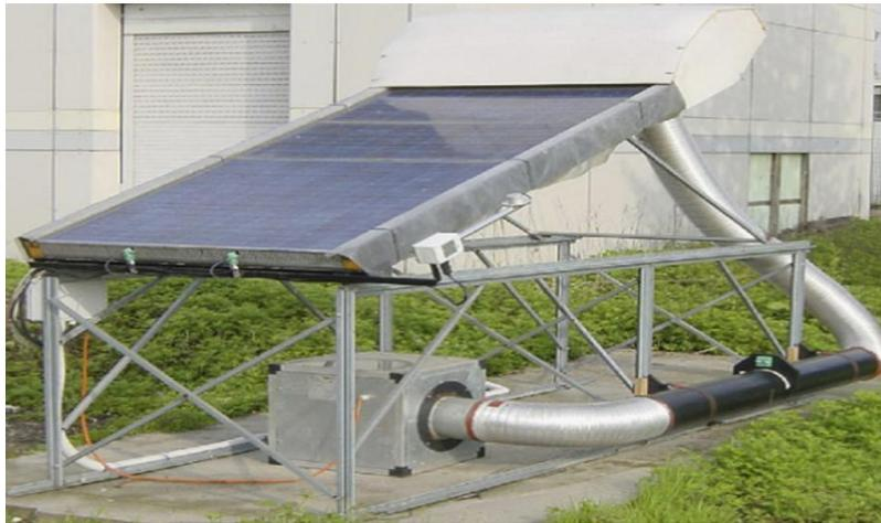
**Fig.9.** A prototype PV/T air collector
