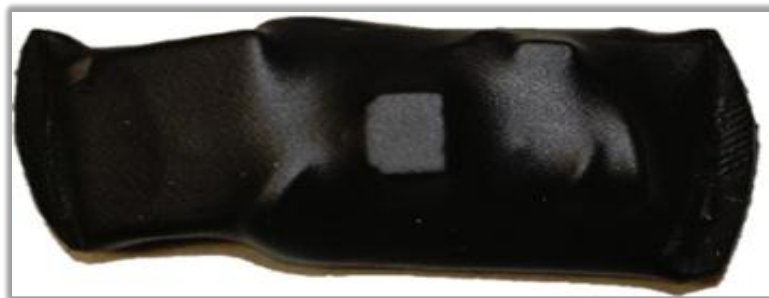
Fig.2. Logger encased in heat shrink tubing for use
