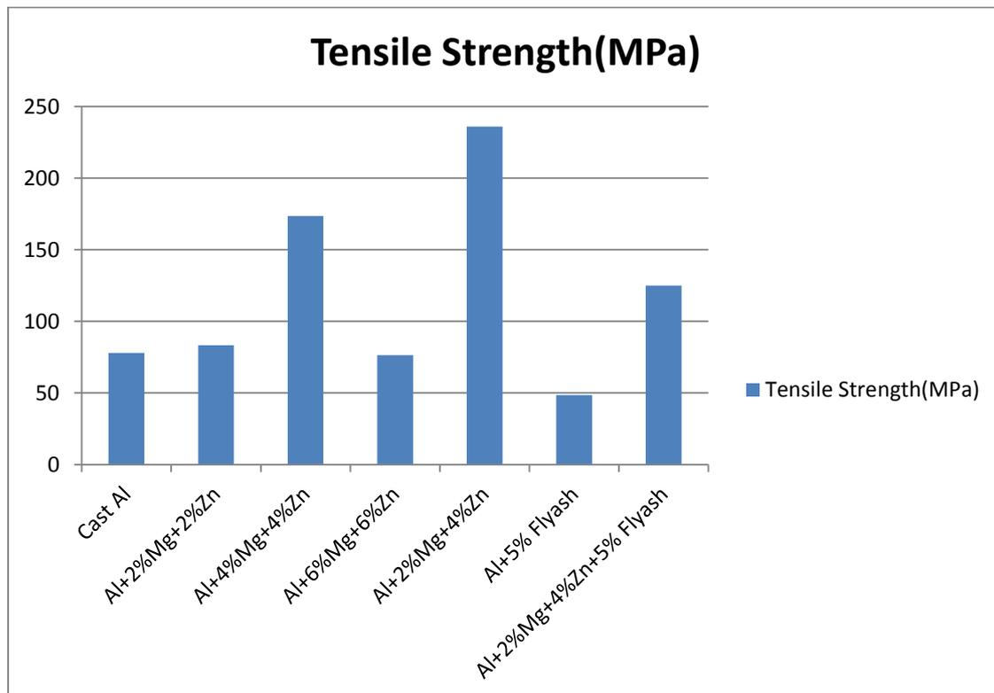
**Fig.(9)-** Graph shows variation in tensile strength with composition of MMC
