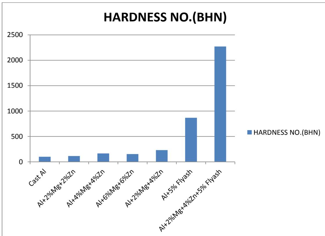
**Fig.(8)** Graph showing variation in hardness with composition of MMCs
