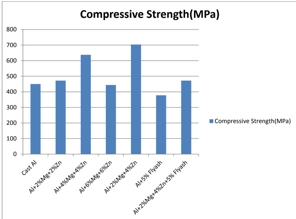
**Fig.(10)-** Graph showing variation in compressive strength with composition of MMC
